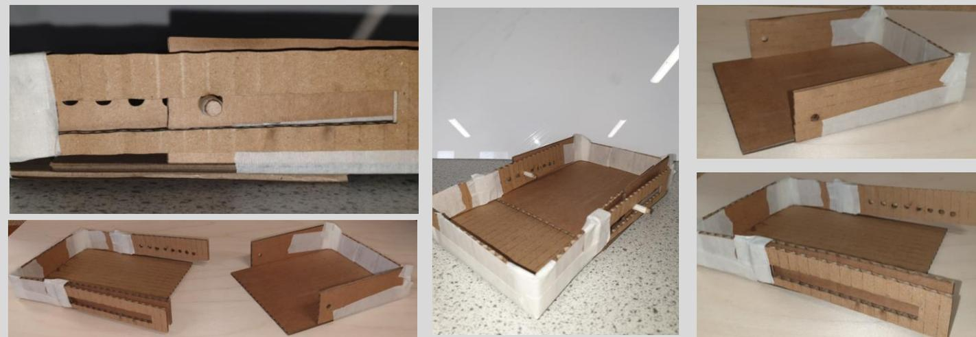
The final net of my packaging is shown below and consists of 14 individual pieces that fit together to create my final iteration model of my idea. The final design model has been manufactured to a scale model of 1cm : 2cm which allows me to explain and present my design without creating too many waste product through the use of too much material.
