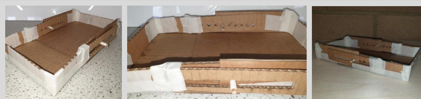
This is the first initial model of my finalised design and as you can see I have introduced the mechanisms that will be used within the assembly. I manufactured this design model using a CAD software programme called 2D Design that allows you to create a net of a design or the different components that will be used. This was then transferred to a laser cutter that cut out the separate components of my design in cardboard before printing my final product in acrylic sheeting.
